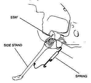
3. Remove the bolt and switch from the side stand.
