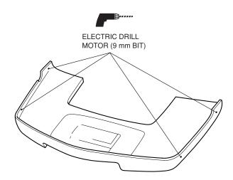
5. Install the trunk rail on the under trunk cover as shown.
