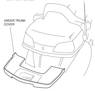
2. Position the template on the **outside** of the under trunk cover as shown. Mark the center of the two dots on the template with an awl. Remove the template.
