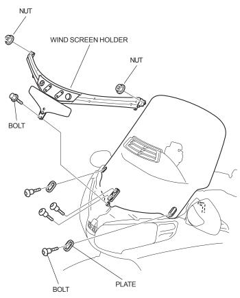
5. Remove the parts from the original windshield.
