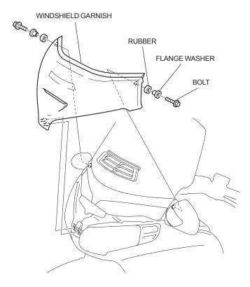
4. Remove the bolts and screws and remove the original screen by pulling it upward in the direction shown.
