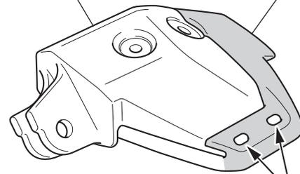
Align the hole of the left wide footpeg cushion with the projected part of the left wide footpeg arm.
