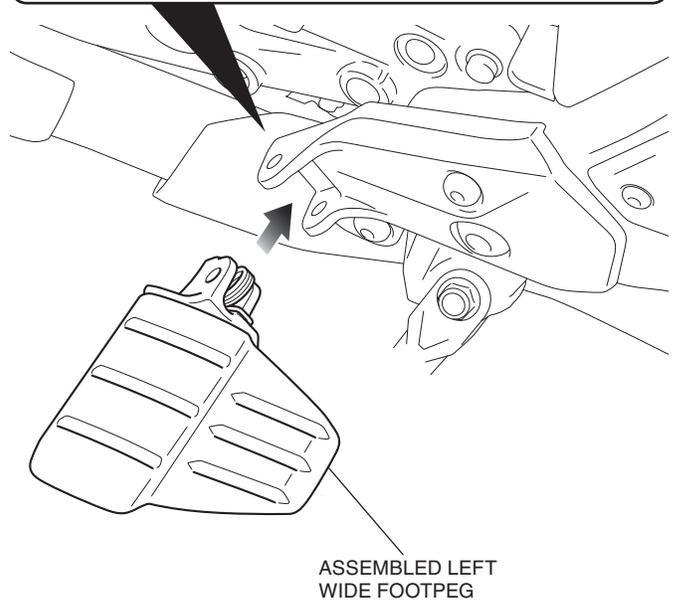
11. Install the pivot pin and split pin as shown.
