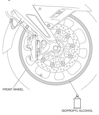
2. Temporarily install the front wheel stripe as shown.
