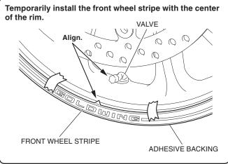
3. Partly remove the adhesive backing from behind the front wheel stripe as shown.
