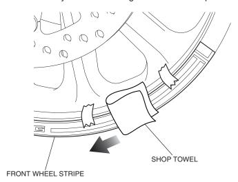
6. Remove the masking tape and application film as shown.
