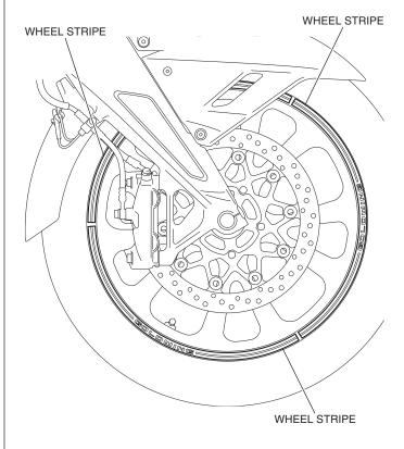
1. Clean the surface of the area shown using isopropyl alcohol.
