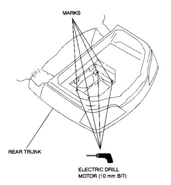
Further locate another mark on the back of the rear trunk and drill a hole through the mark with an electric drill motor and 32 mm hole saw.
