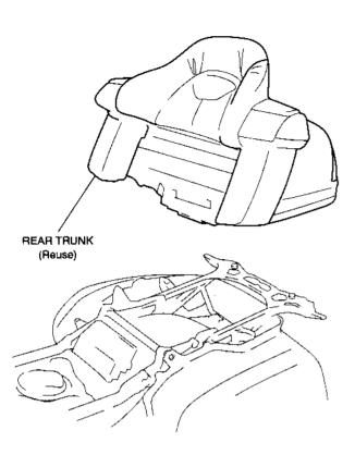
Inside the rear trunk, locate the four marks. Drill a hole through each mark using an electric drill motor and 10 mm drill bit.
