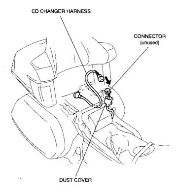
17. Secure the wire harness with the wire tie in the area shown.
