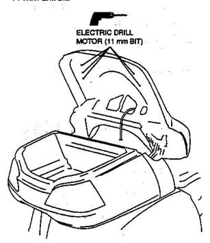
5. Fit the rear spoiler into place on the rear trunk as shown.
