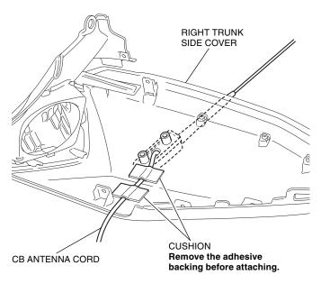
Route and secure the CB antenna cord as shown.Right side>
