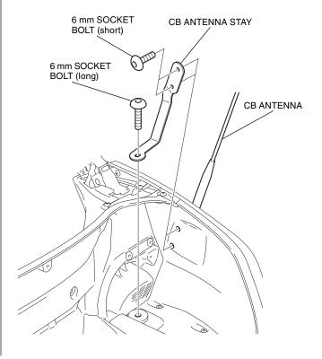
13. Connect the CB antenna cord as shown.
