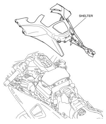
28. Remove the center switch panel as shown.
