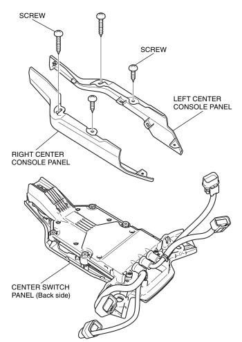
30. Remove the center console garnish as shown.
