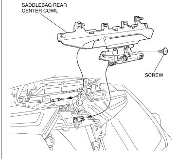
45. Remove the parts as shown.
