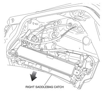
48. Remove the radio antenna as shown.
