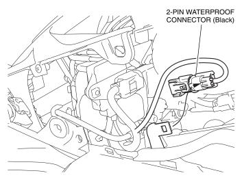
23. Remove the clip and disconnect the connector as shown.
