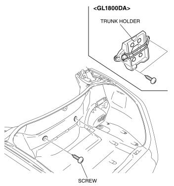
38. Remove the trunk front lower panel as shown.
