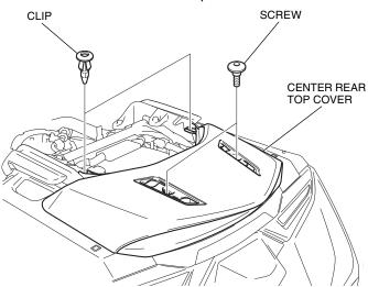
12. Remove the center rear top cover by pulling up and back as shown.
