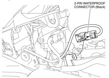
22. Remove the clip and disconnect the 2P black connector as shown.
