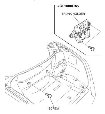
34. Remove the trunk front lower panel as shown.
