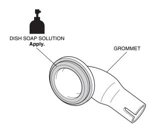
67. Install the grommets at positions shown.
