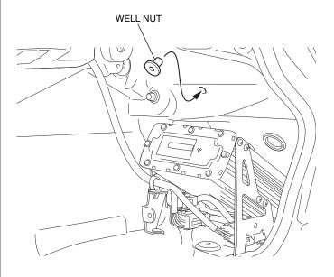
73. Clean the surface of the area shown using isopropyl alcohol as shown.
