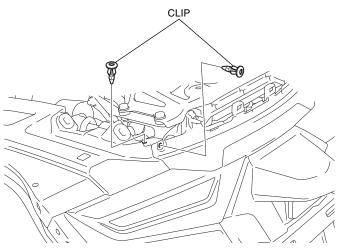
37. Remove the rear fender as shown.
