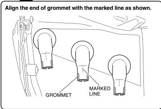
68. Install the hole plug as shown.
