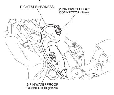
56. Secure the right sub harness with the wire ties as shown.
