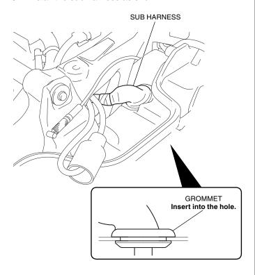
85. Secure the left sub harness with the wire tie as shown.
