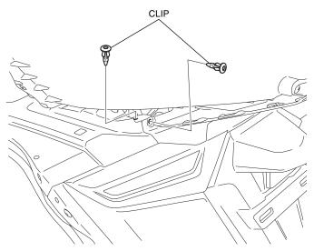
41. Disconnect the connector and remove the trunk center lower cover as shown.
