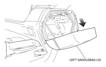
5. Remove the left side cover as shown, and disconnect the battery negative (-) cable.
