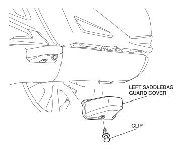
2. Remove the parts as shown.
