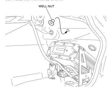
89. Clean the surface of the area shown using isopropyl alcohol.
