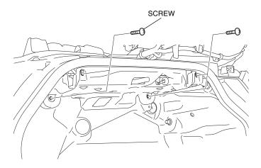
44. Remove the rear fender as shown.
