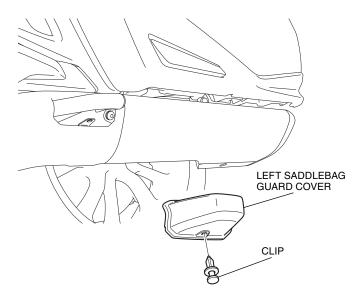
2. Remove the parts as shown.
