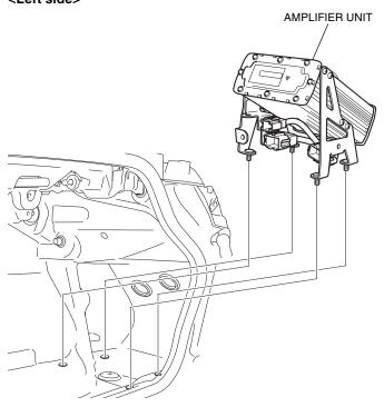
57. Install the 5 mm nuts as shown.
