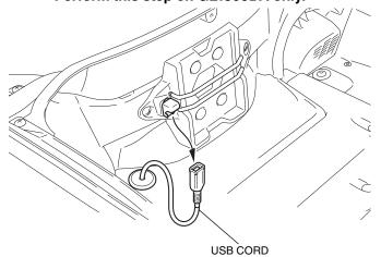
33. Remove the parts as shown.
