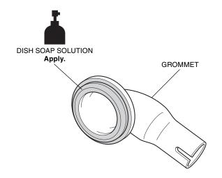
51. Install the grommets as shown.
