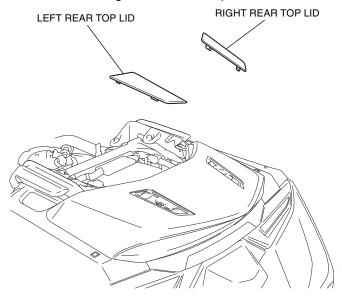
11. Remove the screws and clips as shown.
