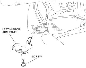
11. Remove the left rear view mirror as shown.
