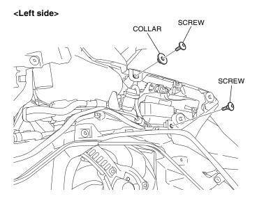
26. Remove the connector as shown.
