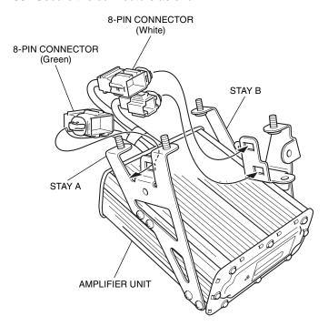
56. Install the amplifier unit as shown.
