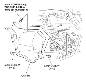
76. Install the 5 mm screw as shown.
