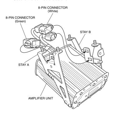
72. Install the amplifier unit as shown.
